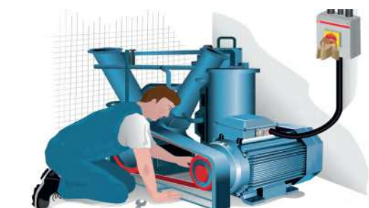
Safety switches protect the operator from unexpected start-up
